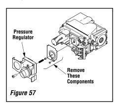
**Step 5.** Attach manometer to the manifold side pressure test fitting and verify manifold pressure reads 3.5 inches water column (0.87 kPa) for natural gas, and 10.0 inches water column (2.49 kPa) for propane gas.
